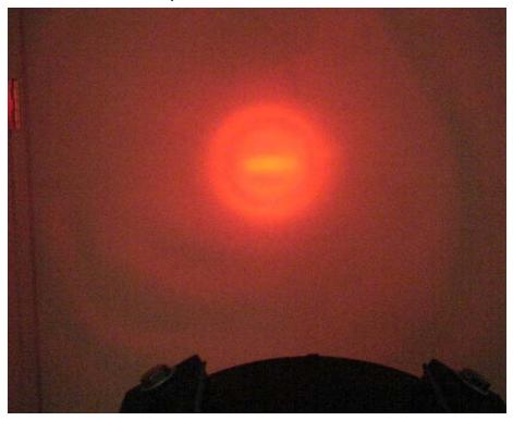
Projected beam pattern at 5-feet without CLS Slide-on Reflector Lamp was 10V25W Lit with 10.0 Volts measured at the Lamp Luminous Intensity Measurement – **462 footlumens**
