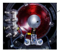
Same S-11 Lamp with the Patent Pending TransLight CLS Slide-on Reflector applied.
